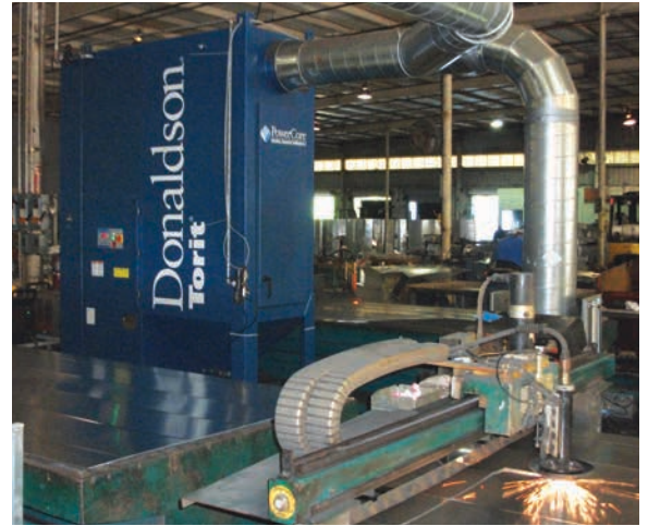
TG on Plasma Cutting 3,400 cfm (5,775 m 3 /h)
