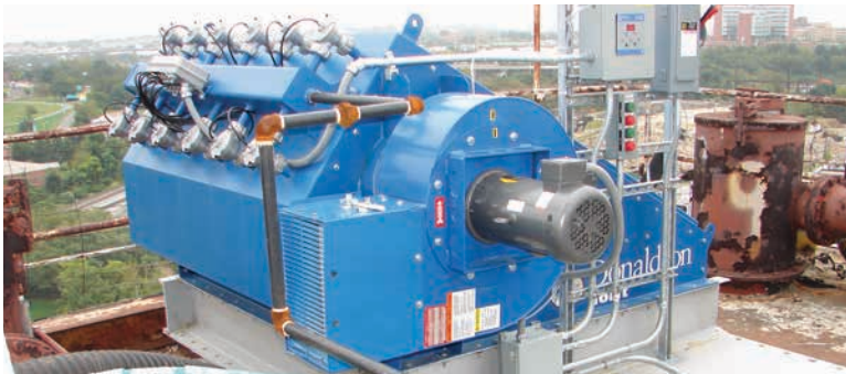
CPV - Multiple Cement Silos 4,800 cfm (8,154 m 3 /h)
