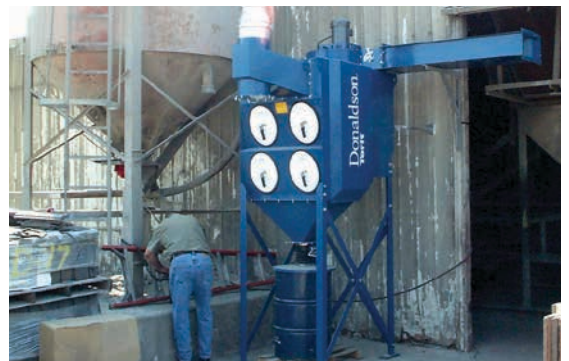
DFO - Concrete Roof Manufacturer 3,000 cfm (5,096 m 3 /h)
