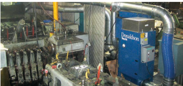
WSO on Cold Forming 1,200 cfm (2,038 m 3 /h)
