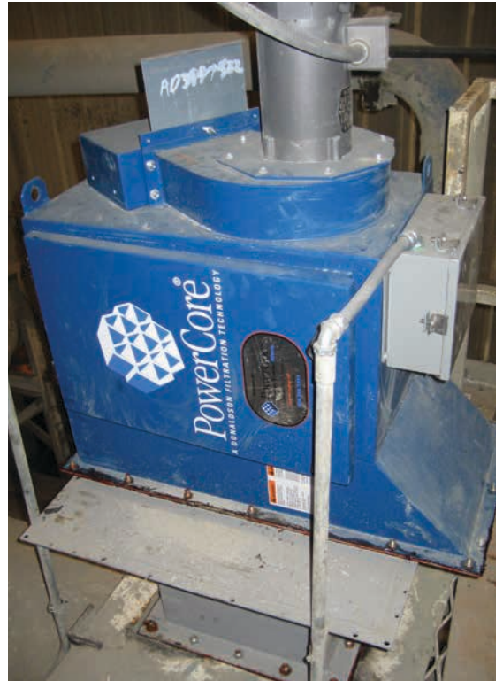
CPV - Feed Hopper 350 cfm (595 m 3 /h)
