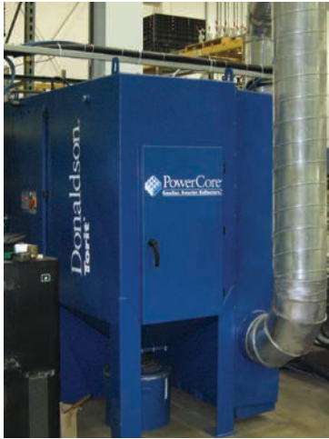
TG on Plasma Cutting 2,300 cfm (3,90 m 3 /h)
