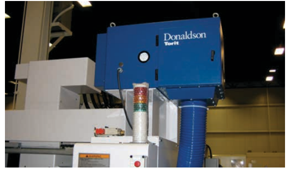
DMC on Wet Machining 390 cfm (662 m 3 /h)
