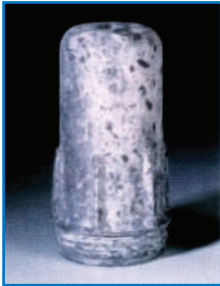
Rapid corrosion of untreated aluminium
